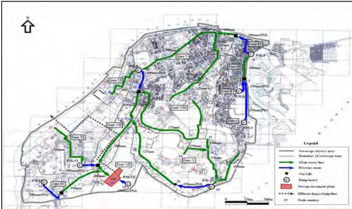
Figure 23.2 General Plan of Panaji Sewerage System
