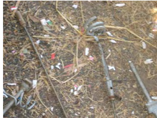
Photo 32.8 Rods to remove the block
