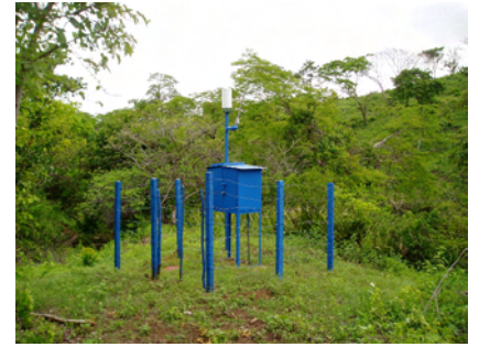
Photo 8-6 Rain Gauge and Telemeter
