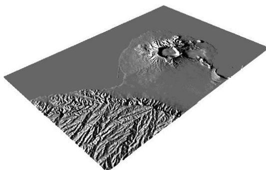
Figure 3-9 Example of 3D shade created from DEM
