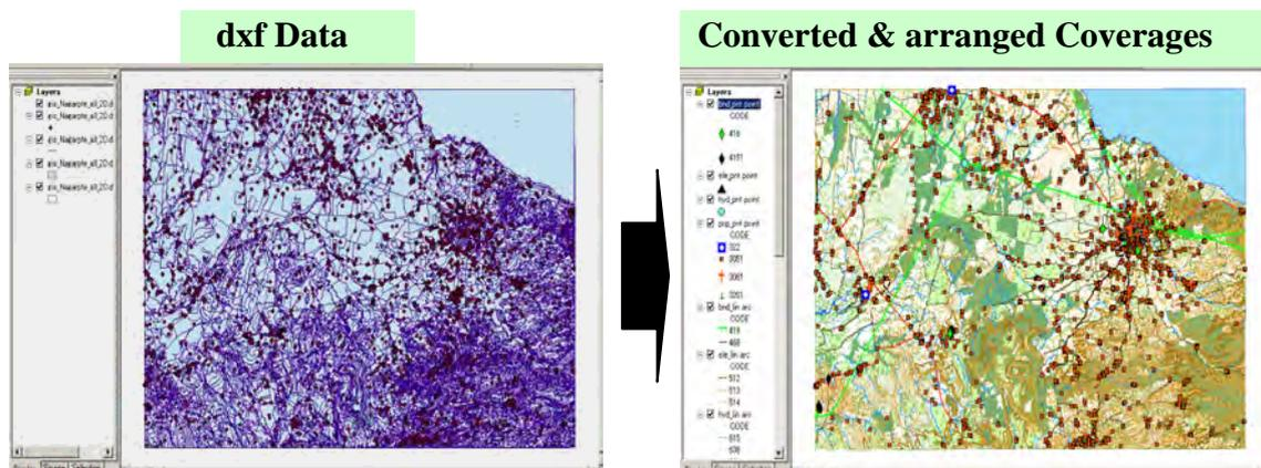
Figure 3-11 dxf Data to Converted and Arranged Coverage Data of 2852-I (Nagarote) Map Sheet
