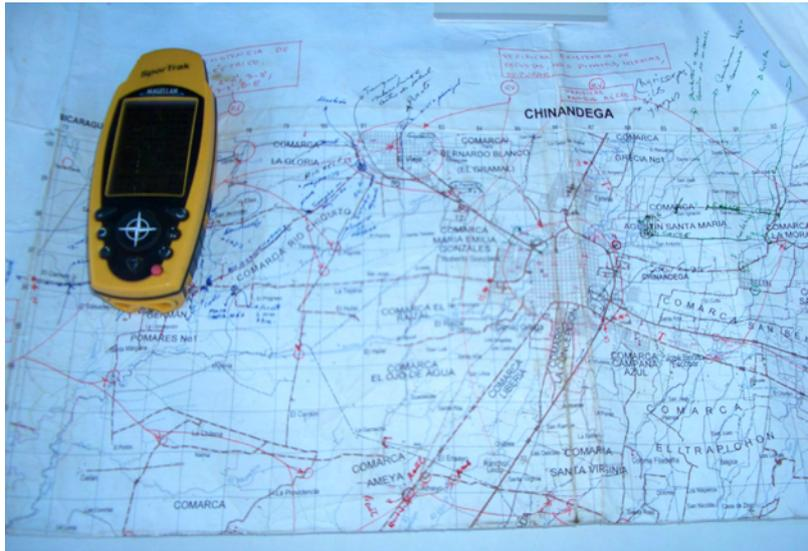
Figure 3-18 Field Completion Map Indicating Coordinates from Handy GPS
