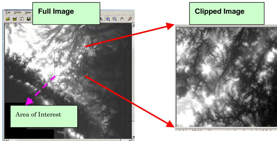
Figure 3-12 Example of Clipping Using an AOI as Clipping File
