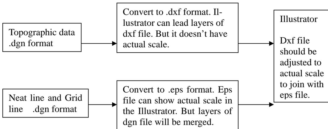
Figure 3-17 Process of Data Format Changes
