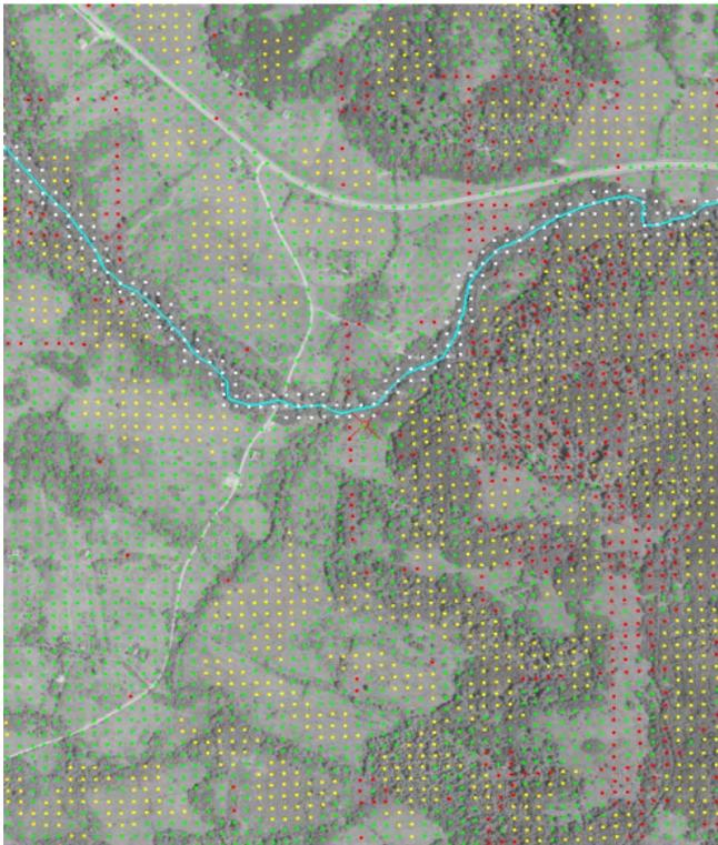
Figure 3-5 Break line and DTM Prepared by Trainees
