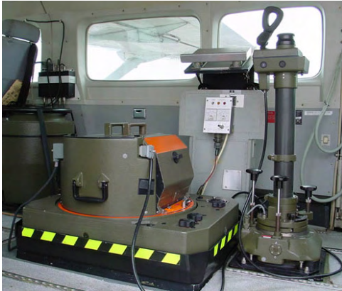
Photo 2-1 Leica RC 30 Aerial Camera
