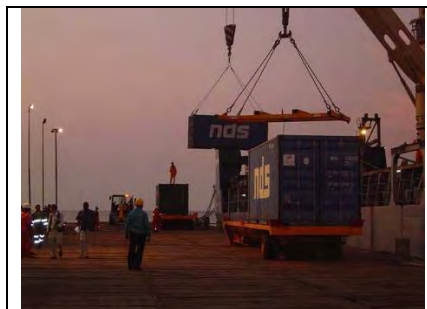
Cargo handling by Mobile Crane
