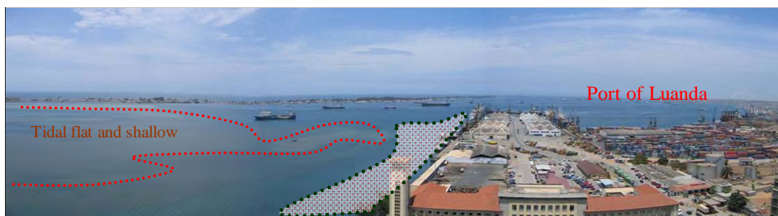
Photo 7-1 Sedimentation in front of Cabotage wharf
