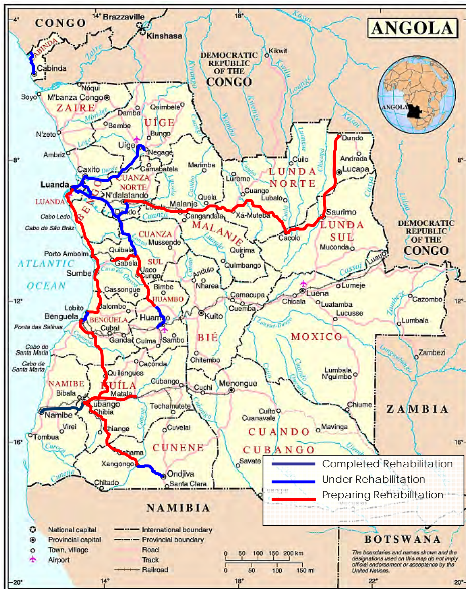
Figure 4-3 Road Rehabilitation in Angola
