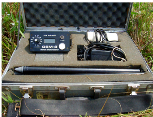
Photo 4.1-2: Magnetic Prospecting Instruments (GSM-8)
