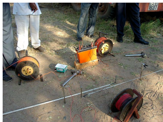
Photo 4.4-1: Electric Prospecting Instruments and Battery
