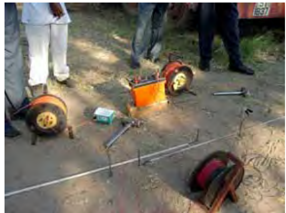
Onsite Technology Transfer (Geophysical Survey: Weirner Method)
