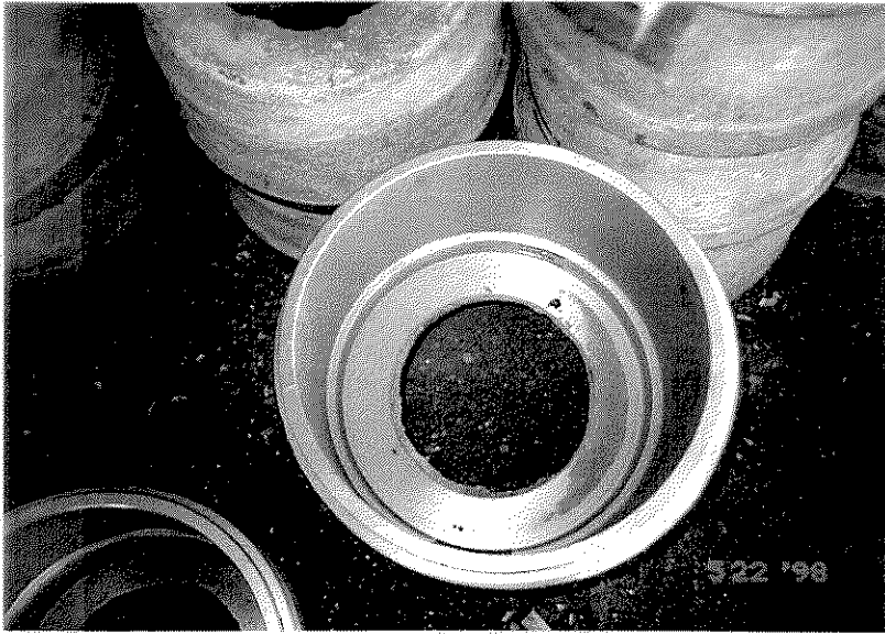
Photo 3-4 Gray cast iron Brake drum for trailers - Casting defects and thickness un-balance are found
