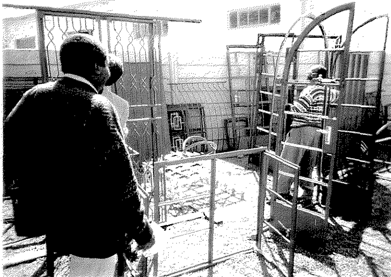
Photo 3-2 Manufacturing of Gates and Window Frame - Individual Production
