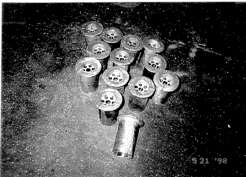
Photo 3-6 Brass part for water sink - Made by gravity die casting - Good shape and cast quality
