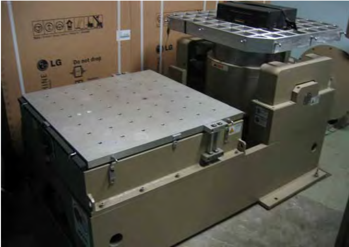
Vibration machine used for checking big appliances (e.g. washing machine) under great pressure. The purpose of this test is to check the capacity of appliance to withstand distant travels during delivery.
