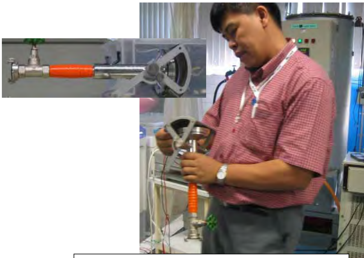
Spray nozzle for uniform application of water to the washing machine
