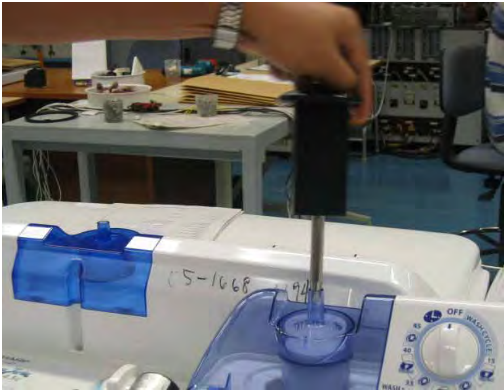
Test finger used to check if appliance conjures electric shock to user.
