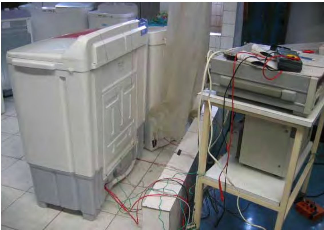
Digital power meter used for testing the watt consumption of washing machines
