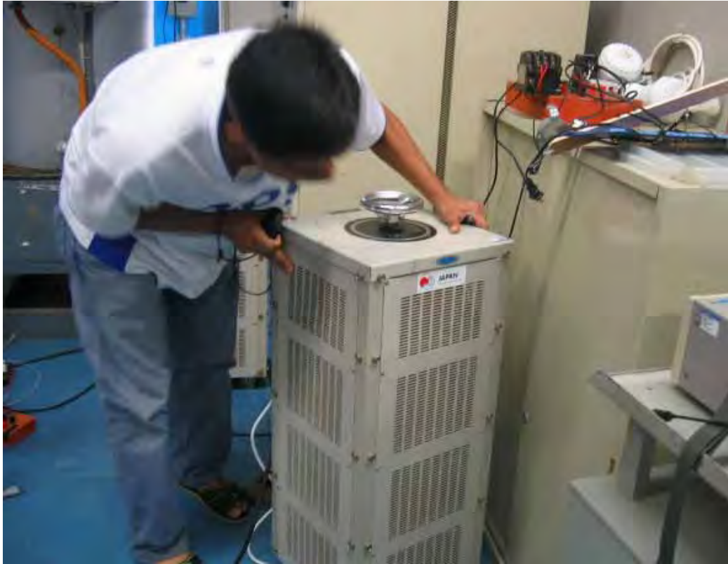
Volt slider used for current/power regulating of washing machine
