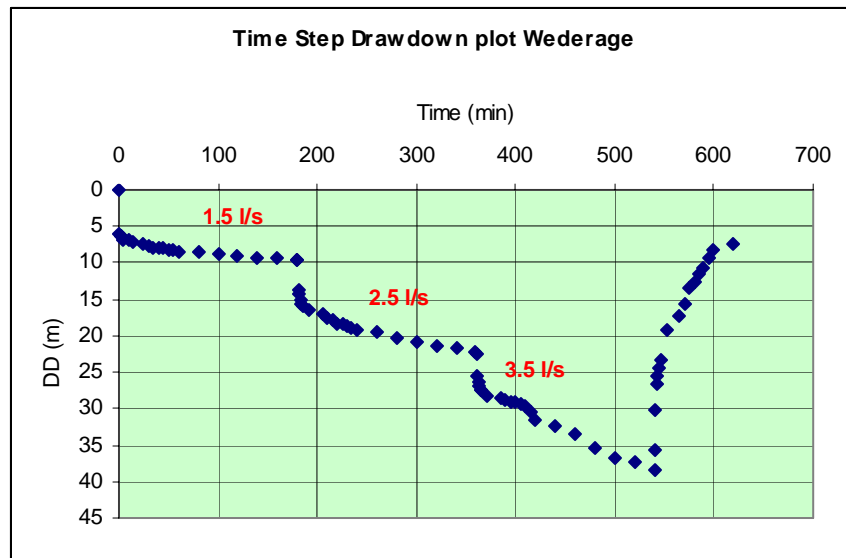
Figure - Wederage Town, Plot of drawdown vs time of the step test
