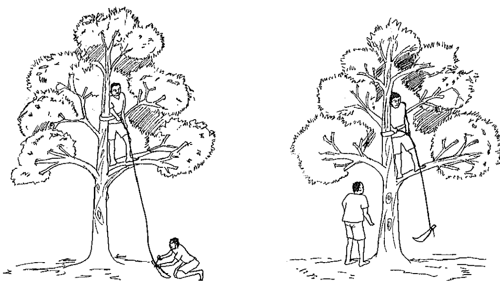
Figure 7.3: Use a light line to hoist any equipment
