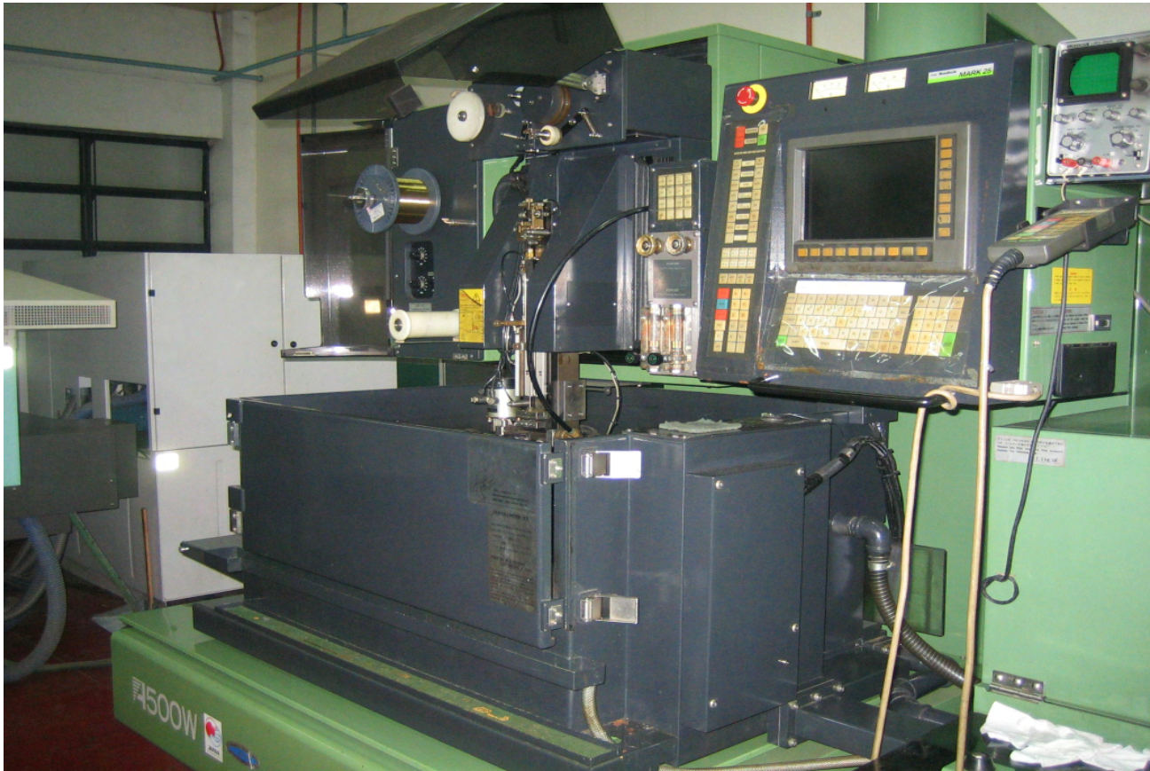
Wire cutting machine supplied to MIRDC by the project
