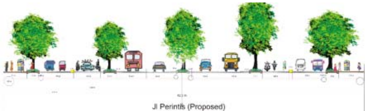
Figure 6.2.1 Typical Section of Proposed Road Improvement
