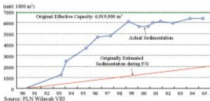
Figure 1.2-8: Sedimentation in Bakaru Reservoir
