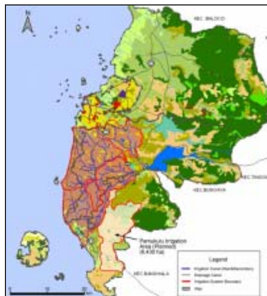
Figure 7.7: Existing Plan of Pamukulu Irrigation Project
