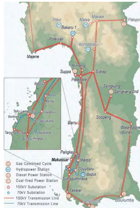
Fig. S-19: Future Transmission Grid
