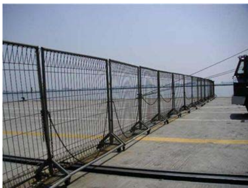
Fence is moved in accordance with the size of restricted area.
