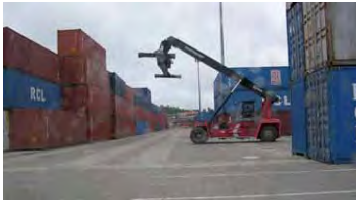
Container handling by a reach-stacker in the yards is carried out .Concrete interlocking blocks are used for the yard
