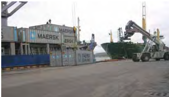
Container handling at the conventional wharf by the vessels own gears and reach stackers.
