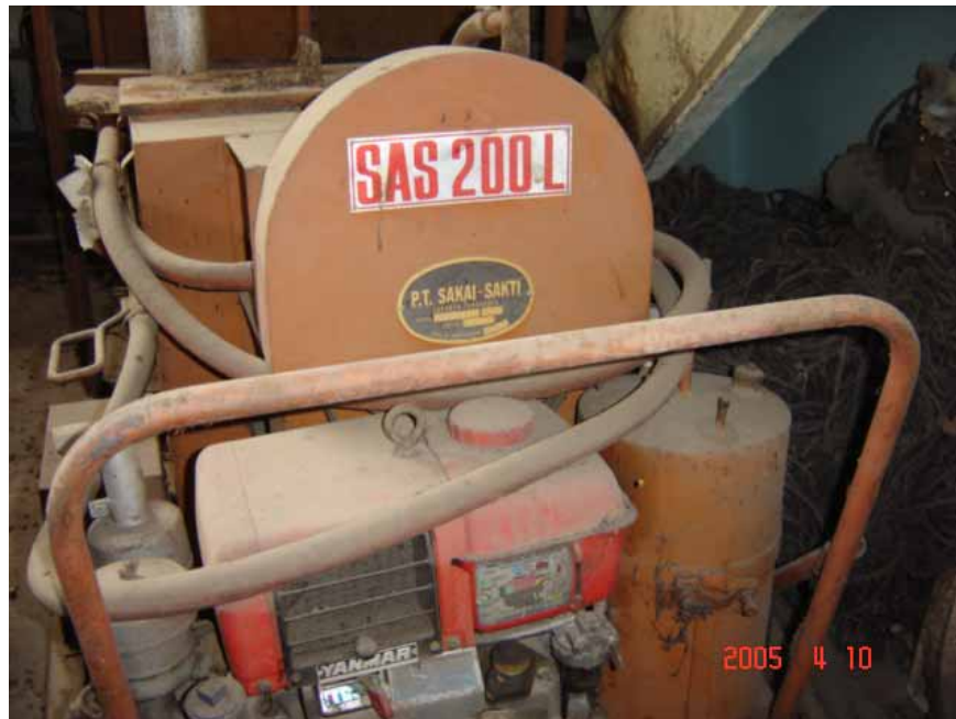
Photograph No. 2. Asphalt sprayer 200 liters rare be utilized, still functioned well at Irrigation Center, Bekasi
