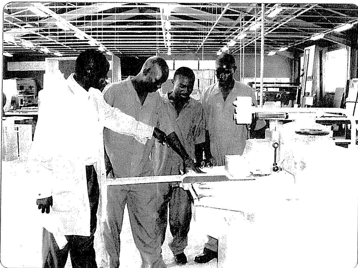
An Instructor guiding the trainees make a precision ripping on a rip saw
