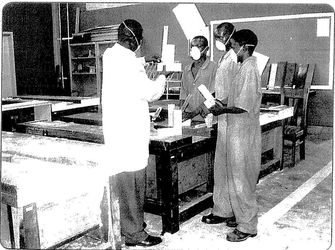
An Instructor demonstrating how to check on the squareness of the module
