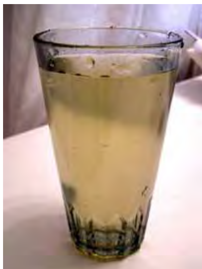
Supplied water coloured by iron
