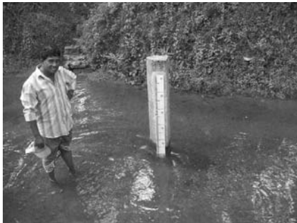
Staff gauge at the head of D-canal at LB Tract 2 in control area (Rajangana)
