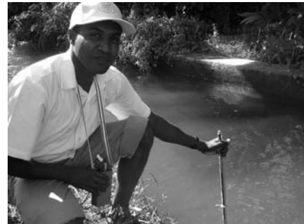
Operation of current meter by Development Assistant (Rajangana)
