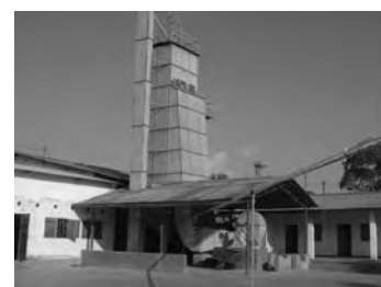
Mechanical Paddy drier, dried by water steam, generated by husk furnace
