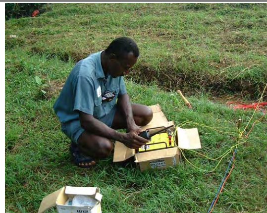
Situation of field work of electric survey. The survey was carried out covering entire Honiara to detect promising aquifer.
