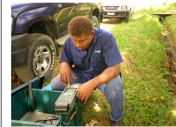
Leakage detection survey done in Phase-1 of this Study Water flow for 24 hours was measured by means of portable ultrasonic flow meter in 12 model districts. Through this measurement, minimum night flow (leakage) and distribution pattern were obtained.
