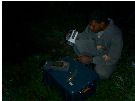
Leakage detection survey done in Phase-1 of this Study SIWA staff is measuring the minimum night flow by means of portable ultrasonic flow meter.
