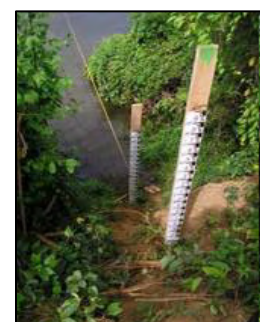
WL Gauging Staff at St.Sanke River, Battambang Province
