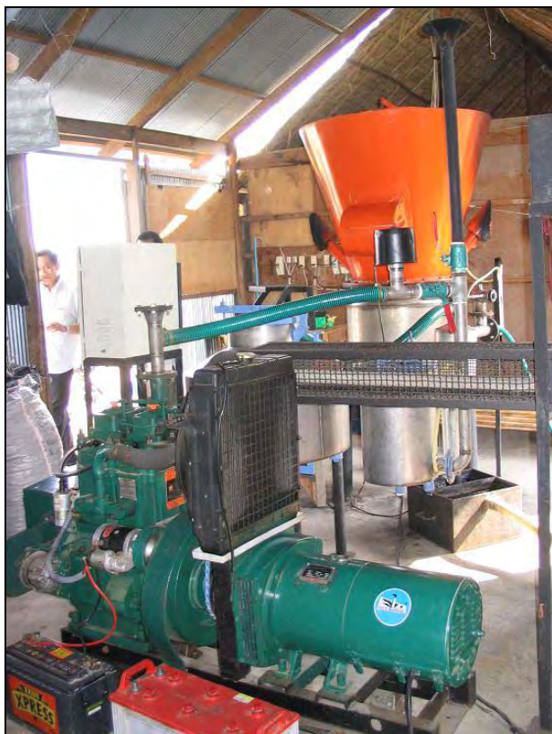
Figure 5.2.5 The 9 kW Woody Biomass Gasifier Installed to Centre for Livestock and Agriculture Development
