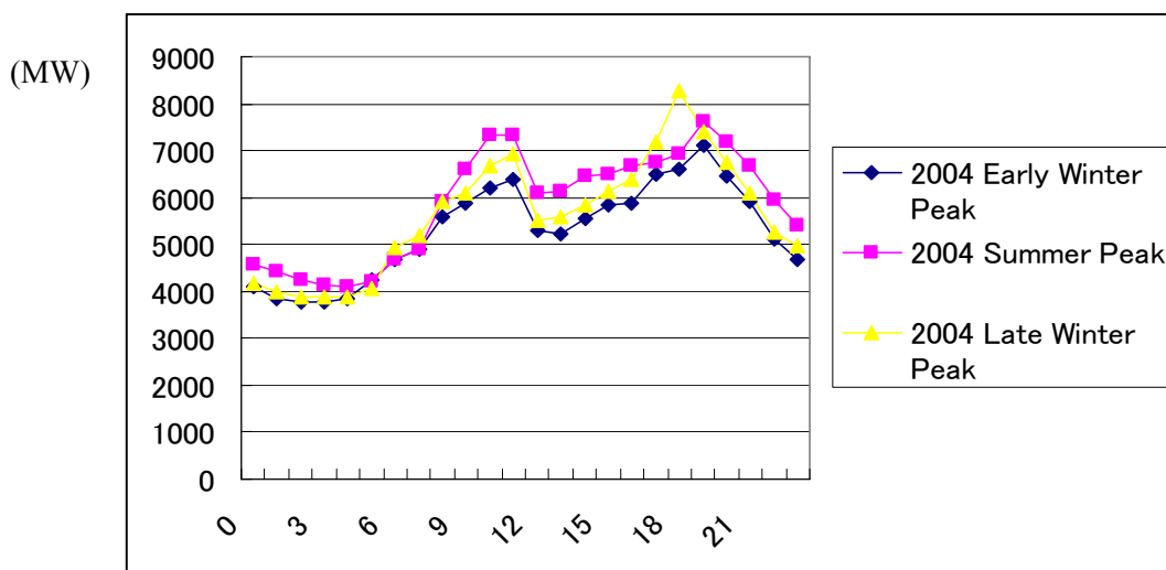
Figure 3-3-11 Actual Daily Load Curve in 2004
