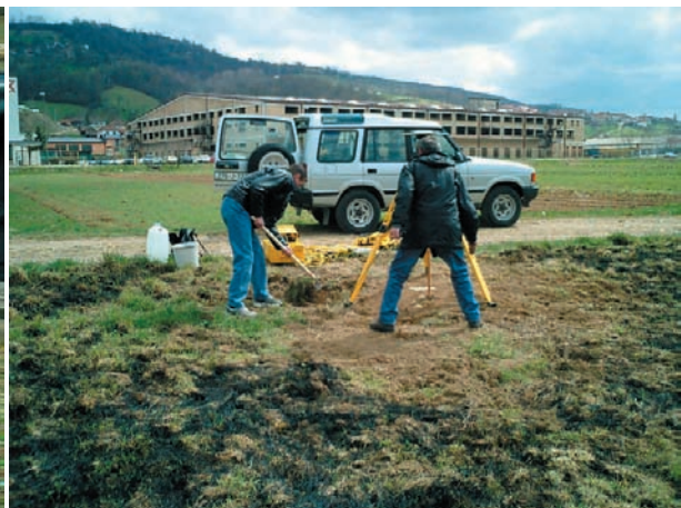
Photo 2 - 8 Signalization of Control Point
