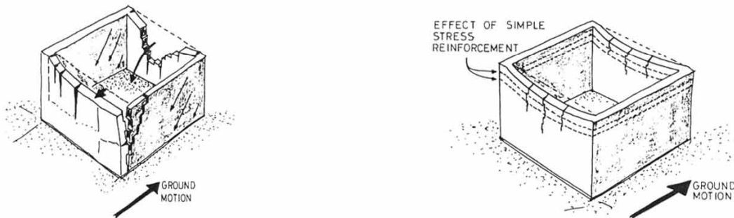
FIGURE 3. EARTHQUAKE FAILURE DUE TO THE BENDING OF A NON-REINFORCED WALL
