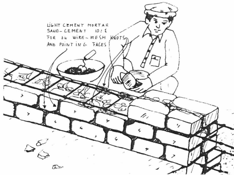
FIGURE 5. THE WIRE-MESH NEEDS TO BE LAID IN SOME MORTAR TO IMPROVE CONTACT WITH THE STONES
