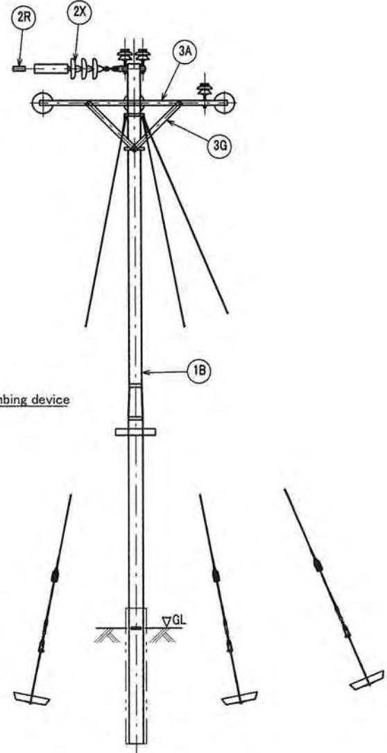
DWG No. DL-E-04: Heavy Angle Pole [ Angle 60 to 90] Pole Type D
