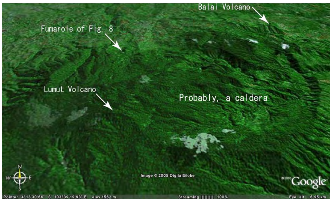
図 3-6 Satellite oblique view of the Lumut Balai geothermal field. A circular topographic area is probably a caldera where white colored spots show alteration zones and steaming grounds. The width of the area reaches 100 km 2 , promising a subsurface enormous geothermal reservoir.
