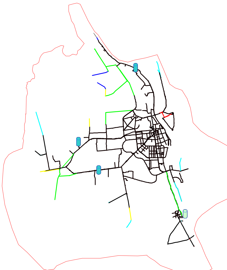
Figure 7-19 Pipes Installed Between 2005 to 2010
