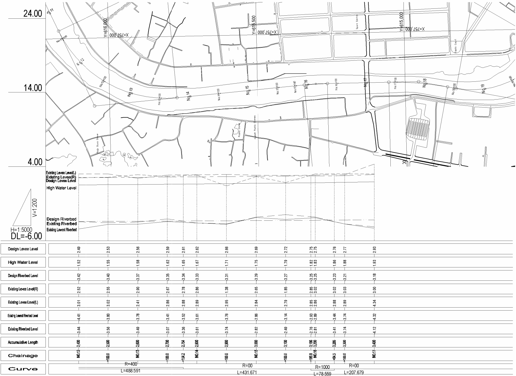
Figure 1.2.8 Plan and Profile of Aech River under Case 2 (3/3)
