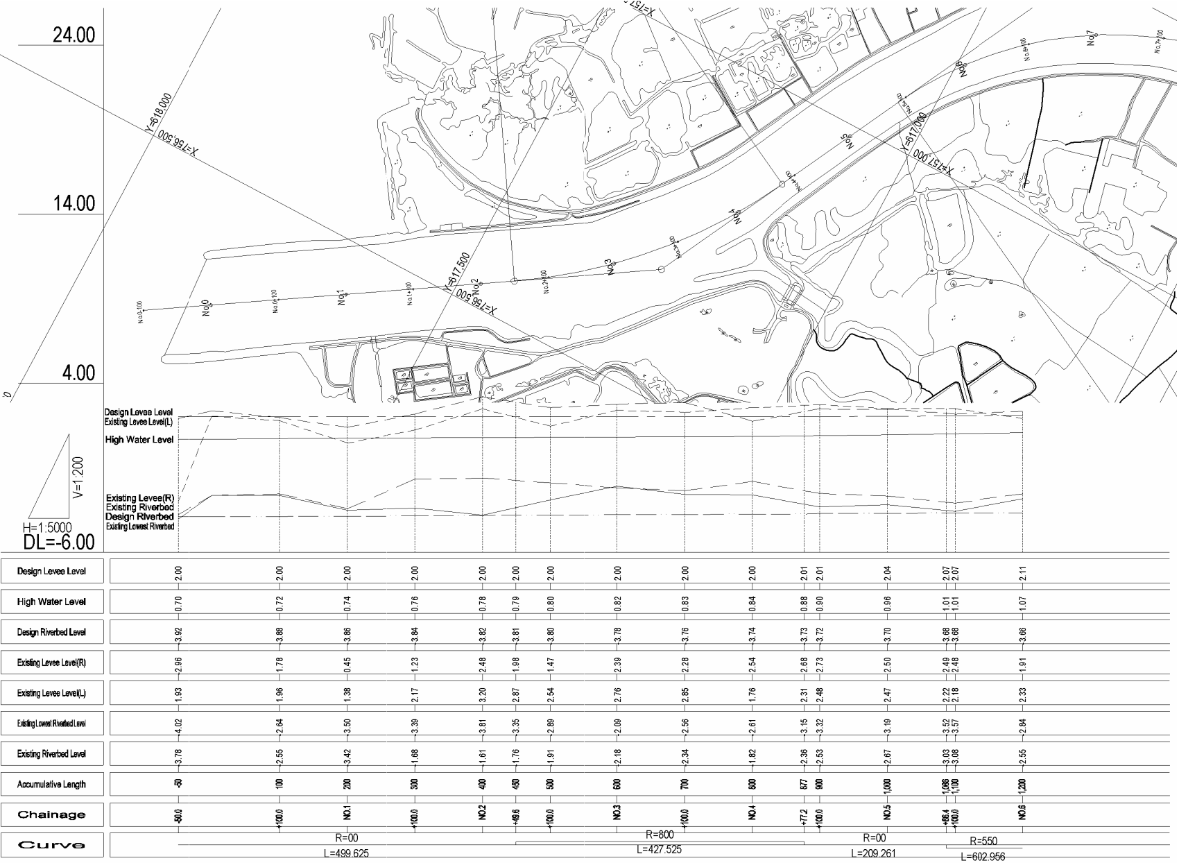
Figure 1.2.8 Plan and Profile of Aceh River under Case 2 (1/3)
