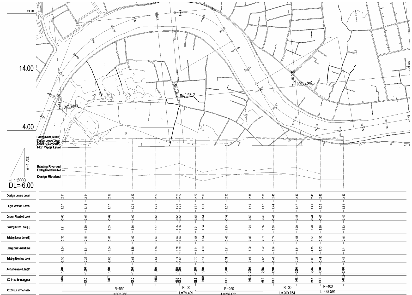
Figure 1.2.8 Plan and Profile of Aceh River under Case 2 (2/3)
