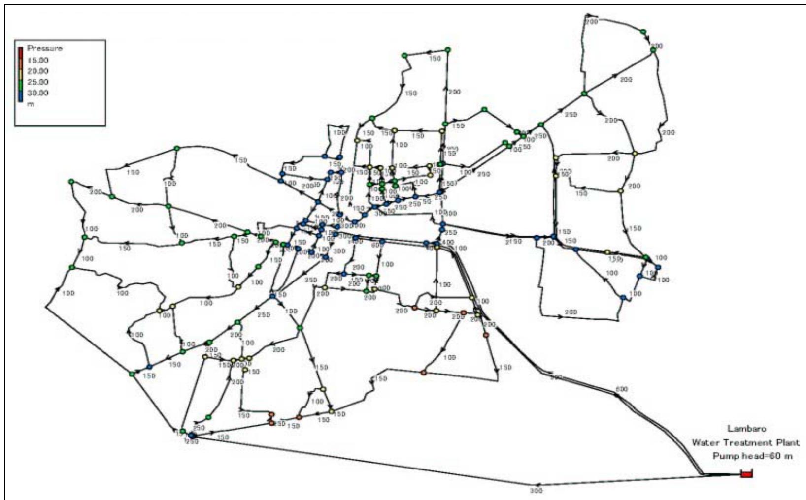
Figure 1.2.4 Result of Hydraulic Analysis, Proposed Restoration Network
