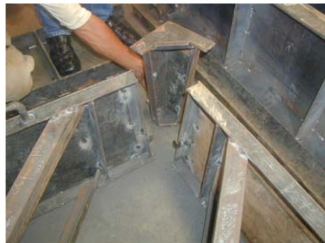
Pre-fabricated concrete for the shaft of khattara
