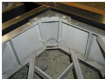
Steel form for pre-fabricated concrete (for vertical shafts)
