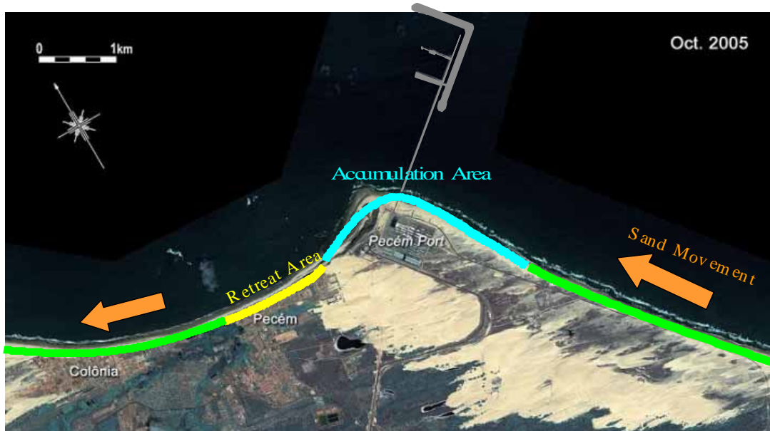
Figure 10.3.1 Impact Caused by the Present Port
