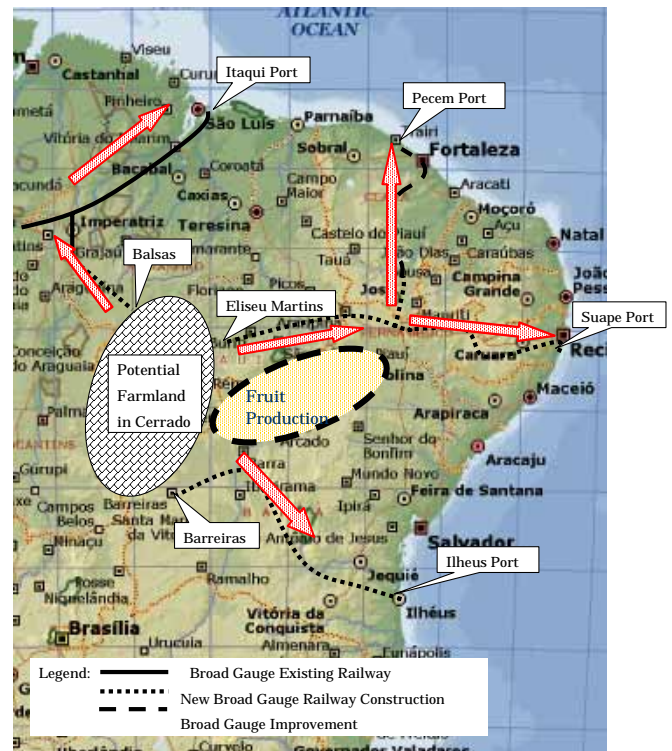
Source: Study Team Fig. 4.10 Railway upgrading Plan
