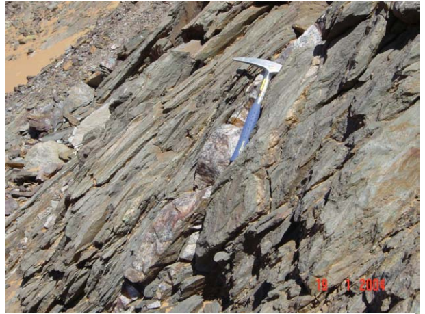
7. Quartz vein (AKM013) with Malachite in Chl. Schist on footwall of Guelb Moghreïn W=10cm, Strike N25W, Dip 42° SW
