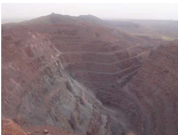
1. Open Pit of Tazadit T01 deposit. Length: 700m (E-W), maximum width 500m (N-S), Depth: 500m
