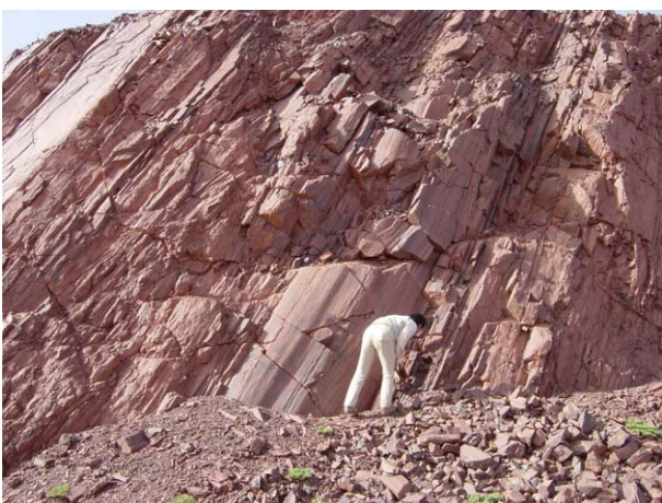
7. Showing Itabrite layer with a low grade of TOI ore body (altitude 680m). Strike 60^\circ W, Dip 55^\circ W
