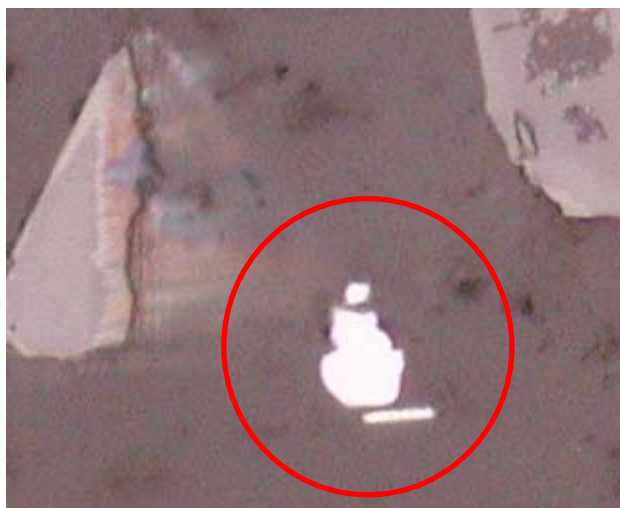
Photomicrograph of platinum group minerals in chromite ore at the Guidimaka deposit
