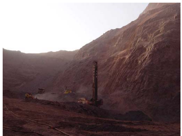
2. Tazadit T014 Deposit. The volume of mining is 19 million tons per year. The ore is composed of hematite with the Fe grade of 45%.
