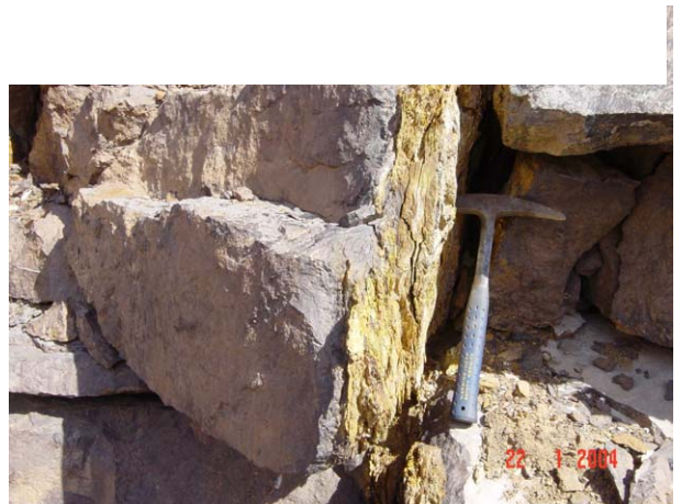
9. Talc vein in Carbonate Ore (AKM018). W=2~6cm strike N48°, dip 90° The abundant anthophyllite is confirmed by X-ray diffraction analysis.
