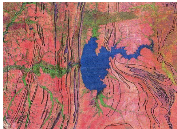
Fig.5.1.2 Draft LANDSAT lineament map of the M'Bout region, Mauritania (Source: British Geological Survey)
