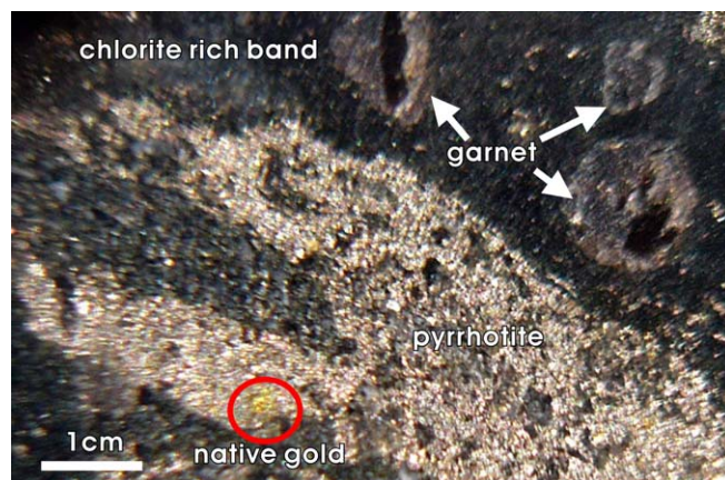
Fig. 4.3.7 Pyrrhotite and native gold with porphyroblast of garnet in chlorite-amphibole band
