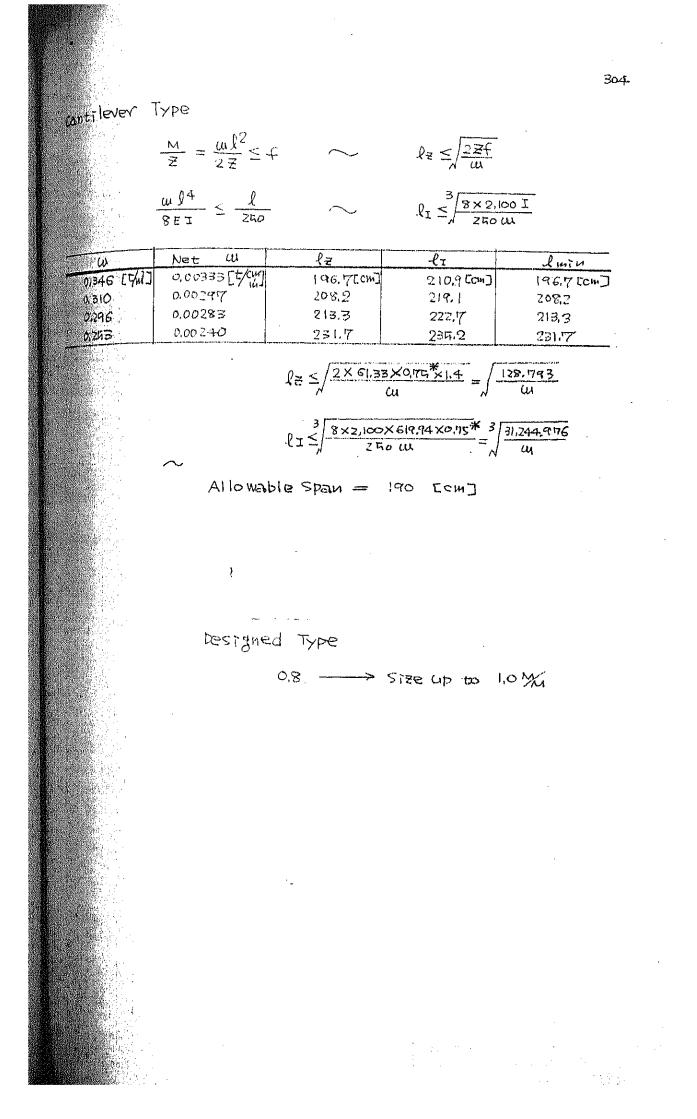
305 lesion of Mezzanine Floor W= 0,71 [ +/m2] 0 - 1.2 Deck Plate Z = 35.5J=136  $\frac{\alpha l^2}{8z} < f \sim l > \frac{8zf}{\omega}$  $= \sqrt{\frac{8 \times 3955 \times 1.4}{9.0051}} = 279.2$ - H W 24 - X 384 EJ - 300 ~ L > / 384 EJ 384×2,100×136 = / = 242.9 100× 0,0051 Allowable Span [CW] 240 - STUD 160 H=100 @ 600 WIRE MESH 100×100×3,2¢ Į SPOT WELDING (0300 (Deck + Beam) V30-300 ( Deck+Deck ) 11 of Furring Strip
