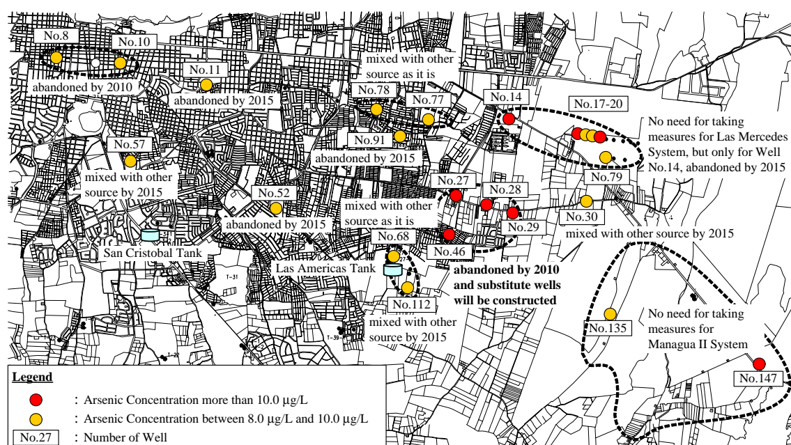
Figure 7.5.12 Measures against Wells having High Arsenic Concentration
