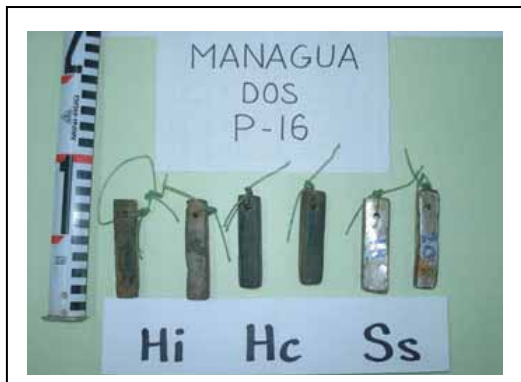
Conditions of Metals (after 2 Months) Hi : Iron Hc : Cast Iron Ss : Stainless Steel
