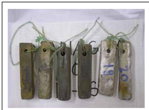
Conditions of Metals (after 2 Months) Hi : Iron Hc : Cast Iron Ss : Stainless Steel
