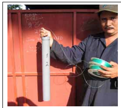
Photo 3.3.2 Measurement unit (PVC pipe) (Oct./2004)
