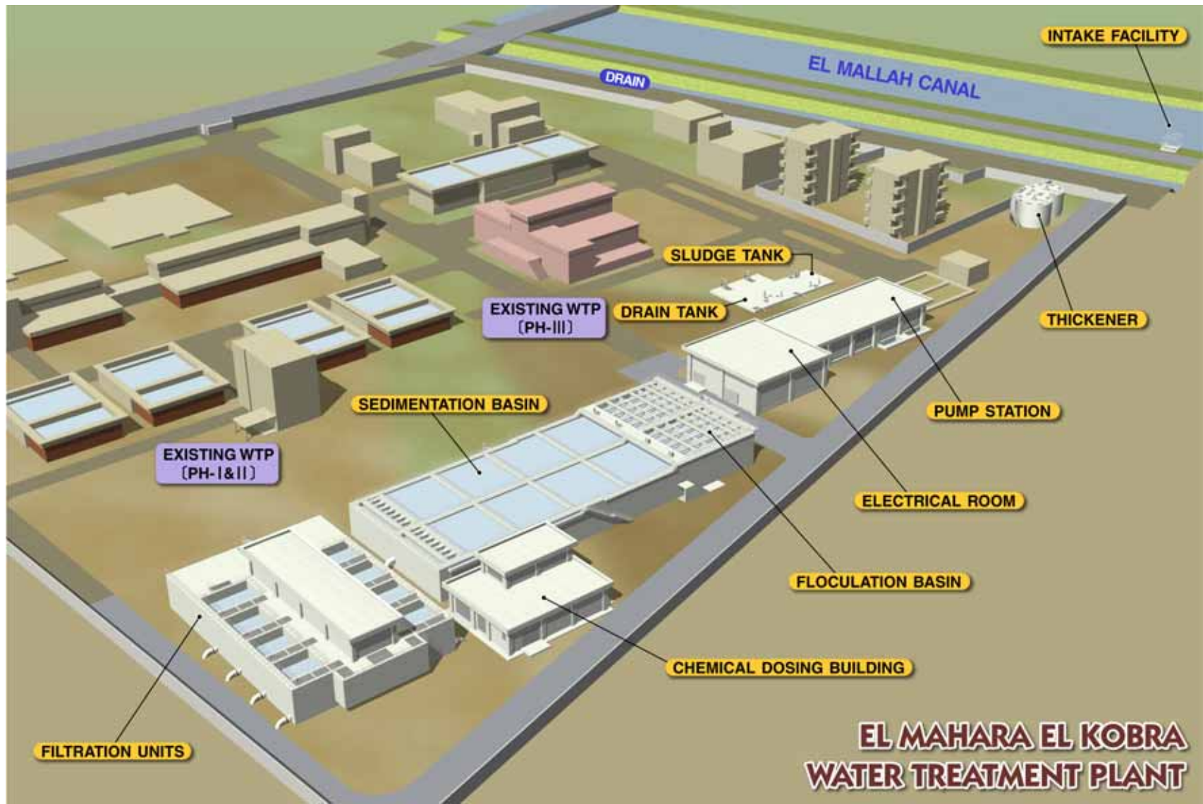
The Perspective of the Water Treatment Plant
